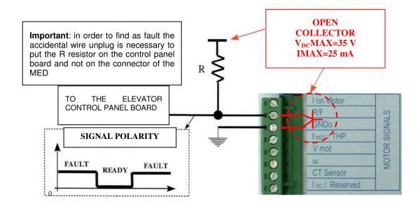
• OPTION n° 2: RELAY CONNECTION (in parallel with the relay coil, connect a suitable wheeling diode)
