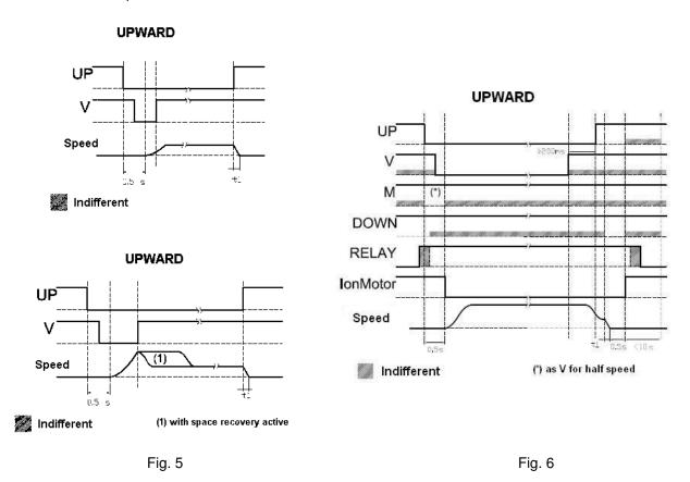
If the signal UP/DOWN goes down when V is still active, the MED executes the S-shape until the positioning speed followed from the t1 slope to stop the motor, independently that it is active or not less the recovery space function. Also in this case the motor power relays must not be opened. If the motor power relays are opened and closed when the commands are present, the MED goes in error A02=ICC-IPM.
